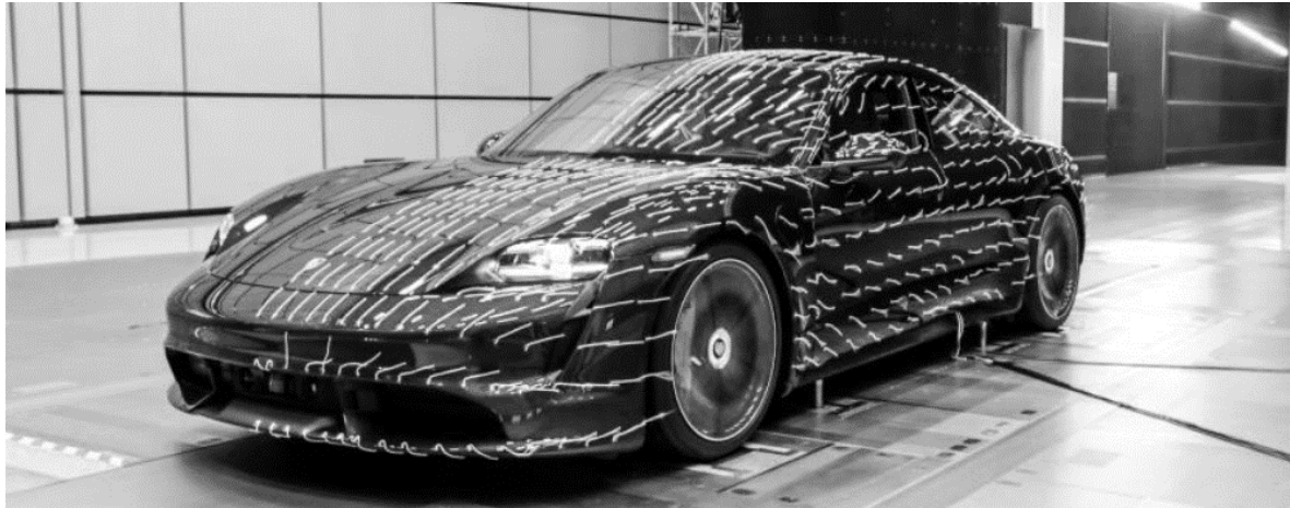
Fig 21: Tuft Visualization method to visualize boundary separation
