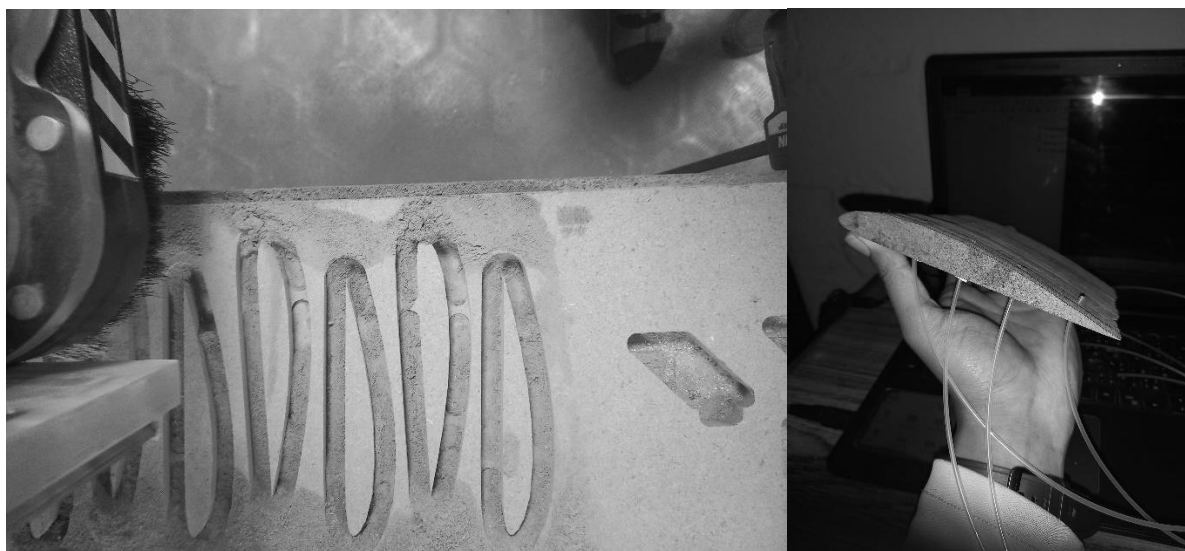
Fig 37: Layer wise manufacture of airfoil profiles using automated CNC
